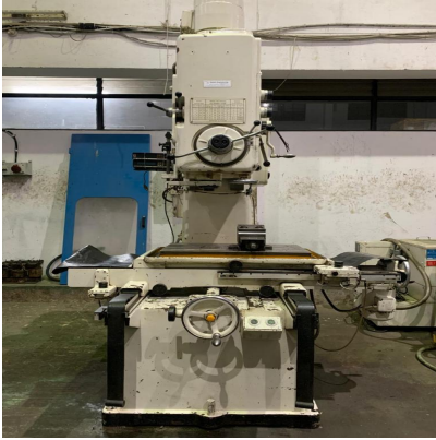
Jig Drilling Machine 650 mm x 400 mm
