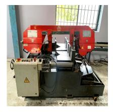
Bandsaw Cutting PPO32 Dia 320 mm
