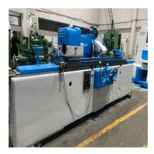
Cylindrical grinding ID-OD MSO 1500 x 250mm
