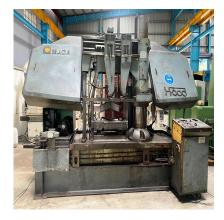
Heavy Duty Band Saw Cutting 600mm
