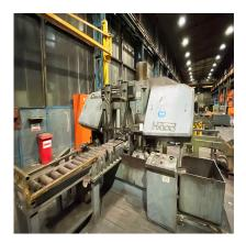
Heavy Duty Single Pillar Horizontal Band Saw 600mm
