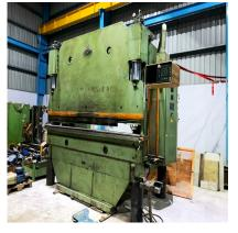
Hydraulic Sheet Bending EHT 3000 x 9mm
