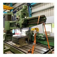
Radial Drilling KOLB 3000 x 85mm
