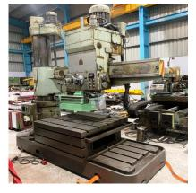
Radial Drilling Stanko 1800 x 70mm
