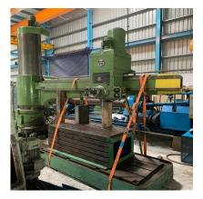
Radial Drilling – WEBO 3200 x 80mm
