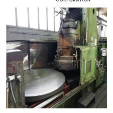
Rotary Surface Grinding 2000mm
