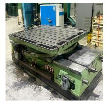
ROTARY TABLE 6 TONS 1900 x 1600mm
