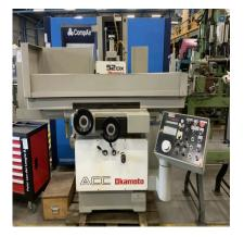
Surface Grinding Okamoto 550 x 200mm
